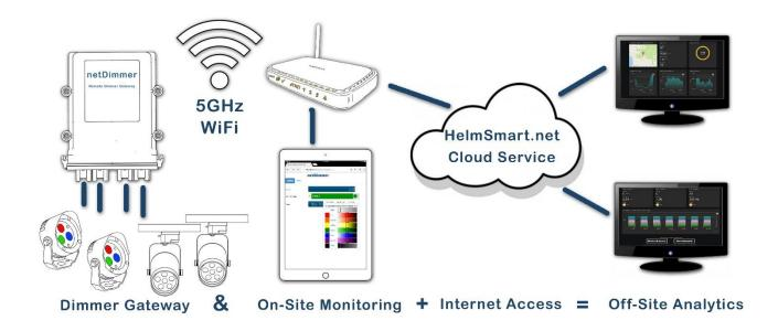
User designed dashboards can be created to view live and historical data in a variety of graphic widgets using any modern web browser device. View current status on your phone/tablet/pc anywhere at any time.
