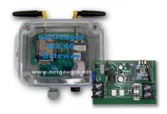
When paired with a netGauges Mesh Gateway, a complete stand-alone closed loop control system can be created. For example, ambient light detected by a netGauges Mesh Gateway can create a command message to be sent over the network to mesh modules to decrease lights levels during daytime.
